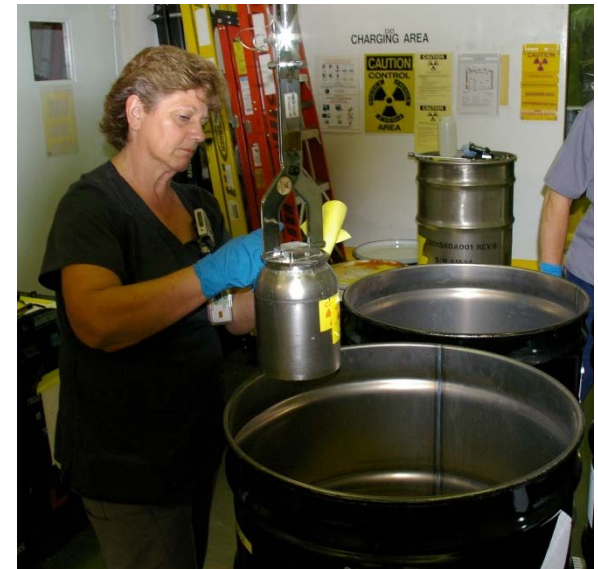
Transferring shielded pigs into ORNL hot cell
