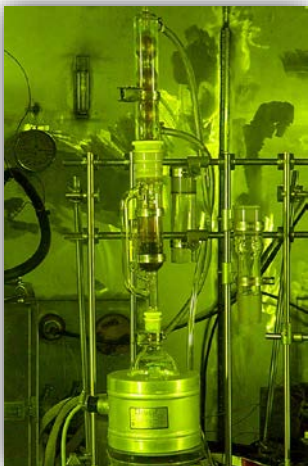
Soxhlet extractor for leach-burn-leach (LBL)
